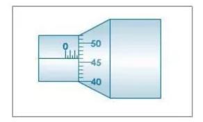
The pitch of the screw = 1 mm L.C. of screw gauge = 0.01 mm Main scale reading = 2.5 mm 46th division of circular scale coincides with the base line. Therefore, circular scale reading =  $46 \times 0.01 = 0.46$  mm Total reading = Main scale reading + circular scale reading = (2.5 + 0.46) mm = 2.96 mm
