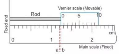
In this position, the zero mark of the vernier scale is ahead of 1.2 cm mark on main scale. Thus the actual length of the rod is 1.2 cm plus the length ab (i.e., the length between the 1.2 cm mark on the main scale and 0 mark on vernier scale).
