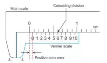
To find this error, we note the division of the vernier scale, which coincides with any division of the main scale. The number of this vernier division when multiplied by the least count of the vernier callipers, gives the zero error.
