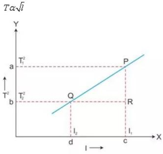
From this graph, the value of acceleration due to gravity (g) can be calculated as follows. The slope of the straight line can be found by taking two points P and Q on the straight line and drawing normals from these points on the X- and Y-axis, respectively. Then, the value of T2 is to be noted at a and b, the value of I at c and d. Then,
